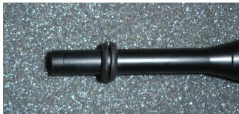
Figure 5. Microphone with 9/32" grommet sound seal used to seal microphone inlet while using Reed SC-05 calibrator
